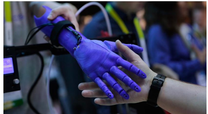
3D printed hand produced on the Intel stand thanks to 3D scan taken using RealSense Technology. Image sourced from m.tech.firstpost.com
